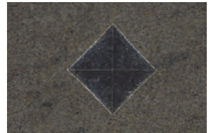
Imprint of a hardness test point
